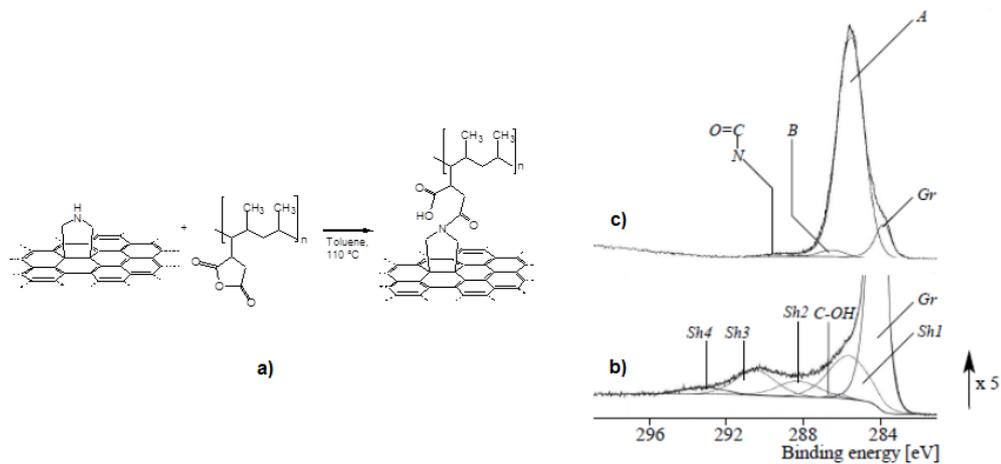
**Figure 1.** CNT functionalization products: a) reaction of the pyrrolidine groups with the maleic anhydride grafted on PP-g-MA; XPS high-resolution C 1s spectra acquired from: b) unmodified CNTs, and c) CNT250/PP-g-MA. The intensity of the spectrum presented for c) is fivefold that of spectrum b).
