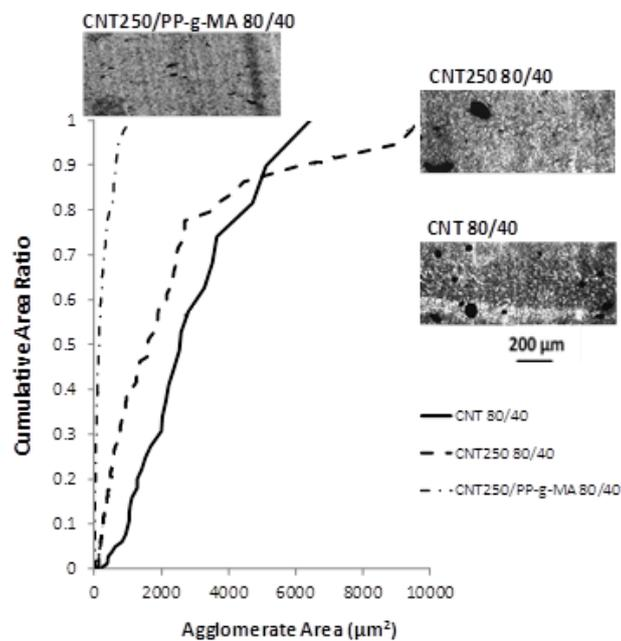
**Figure 2.** Comparison of the cumulative agglomerate area ratios measured for composites processed at 80 rpm and 40 g/h. The insert optical micrographs illustrate the agglomerate dispersion attained.
