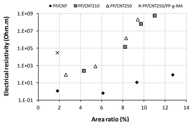
**Figure 3.** Correlation between agglomerate area ratio (ratio between the composite area covered by CNT agglomerates and the total composite area analyzed) and electrical resistivity for composites with 4 wt% of as-received and functionalized CNTs produced under various processing conditions.
